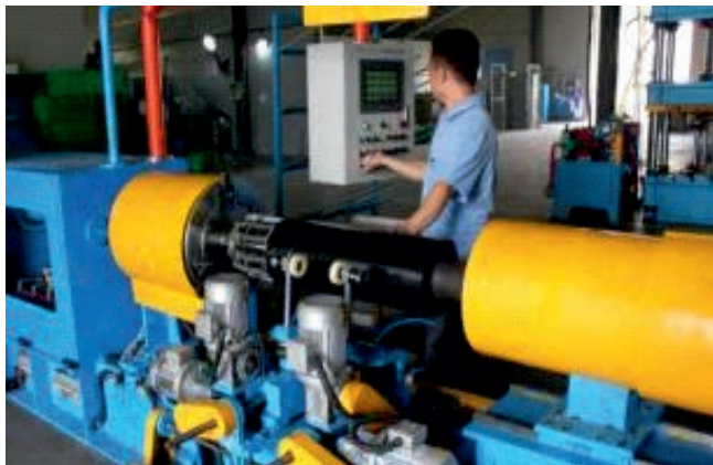
Maszyna do Formowania Gumi / Building for Rolling Lobe Type for Chassis Suspension
